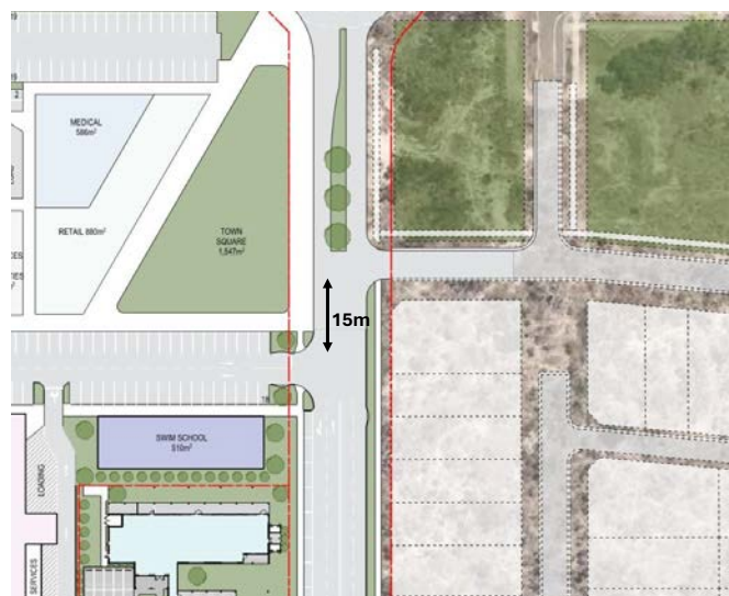
Figure 14: Staggered intersection proposed on the new road
