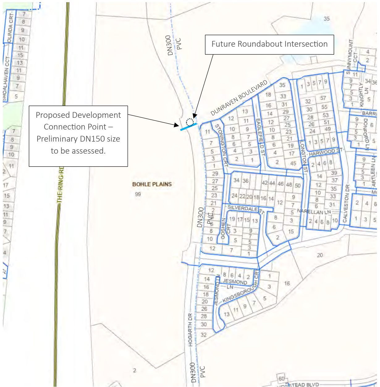
Figure 5: Water Network Mains near Proposed Development Site & Connection Point
