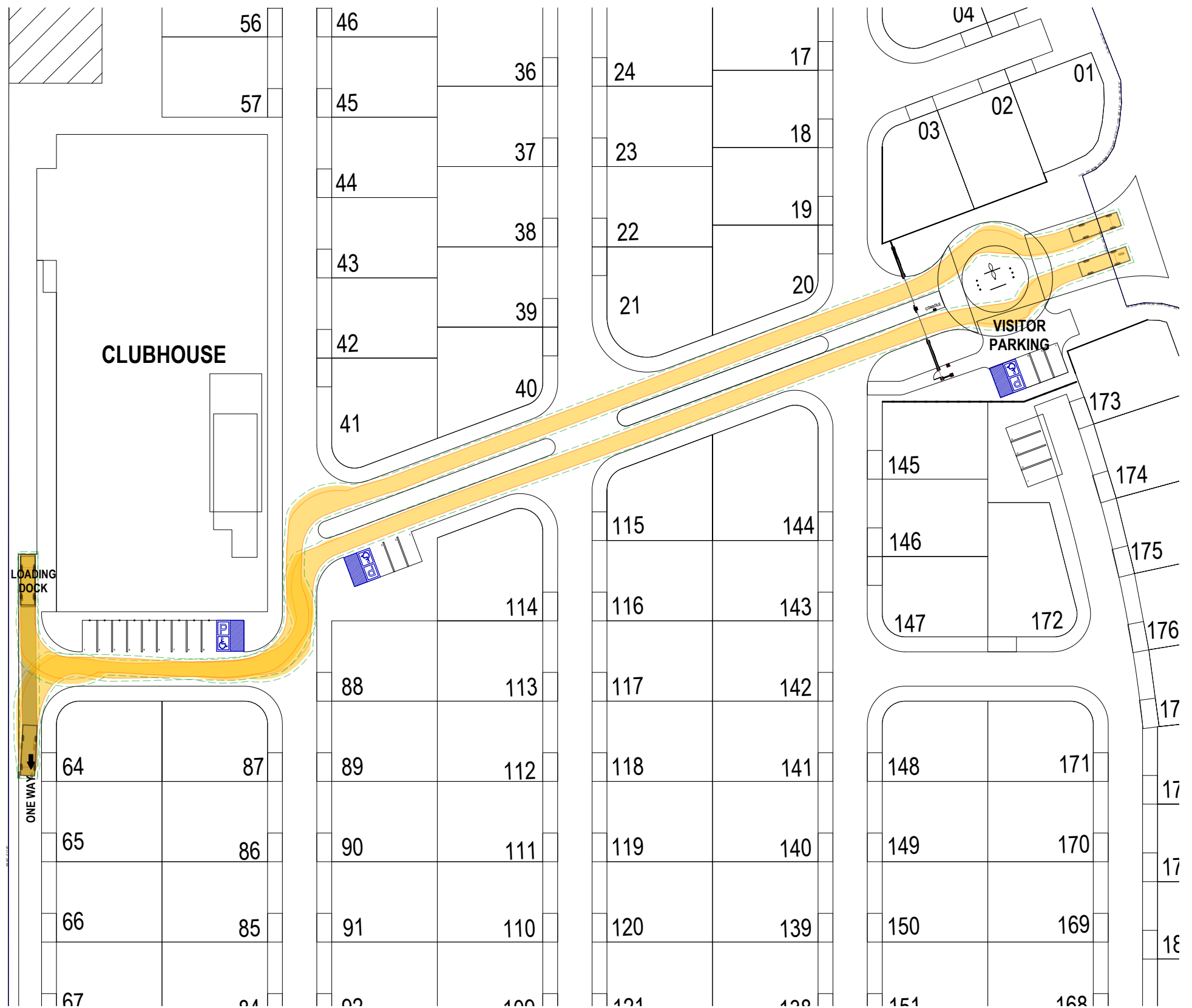
ACCESS TO / FROM CLUB HOUSE LOADING DOCK - MRV REVERSE IN / FORWARD OUT
