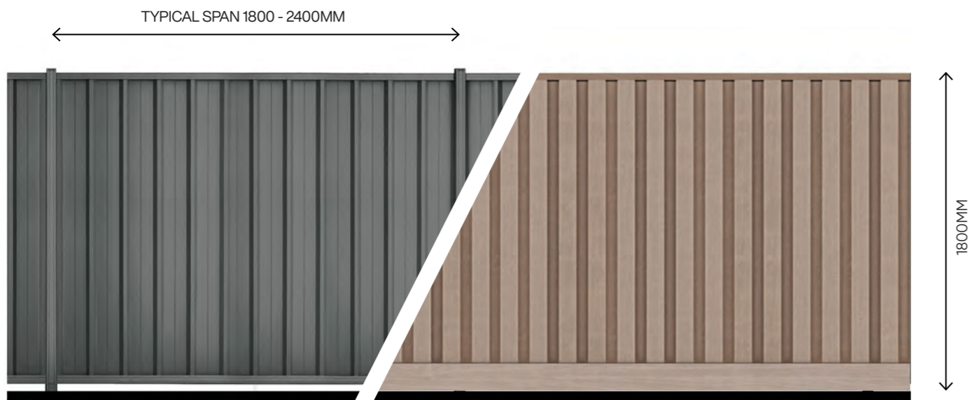
Fence Type B: Typical Elevation
