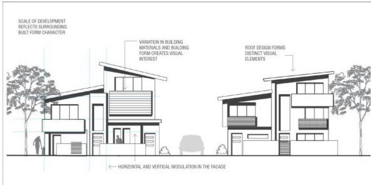
Figure 6.7 Building design elements
