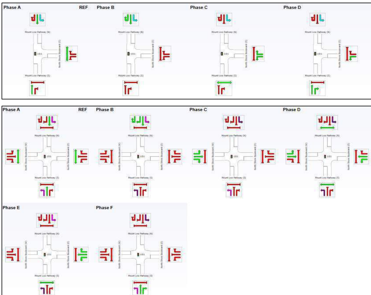
Figure 4.3: North Shore Boulevard / Mount Low Parkway | Ultimate SIDRA Signal Layout
