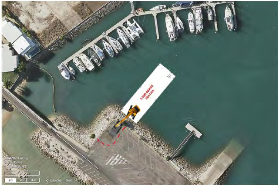
Planned barge unloading location. Red dotted line is planned temporary fencing enclosure
